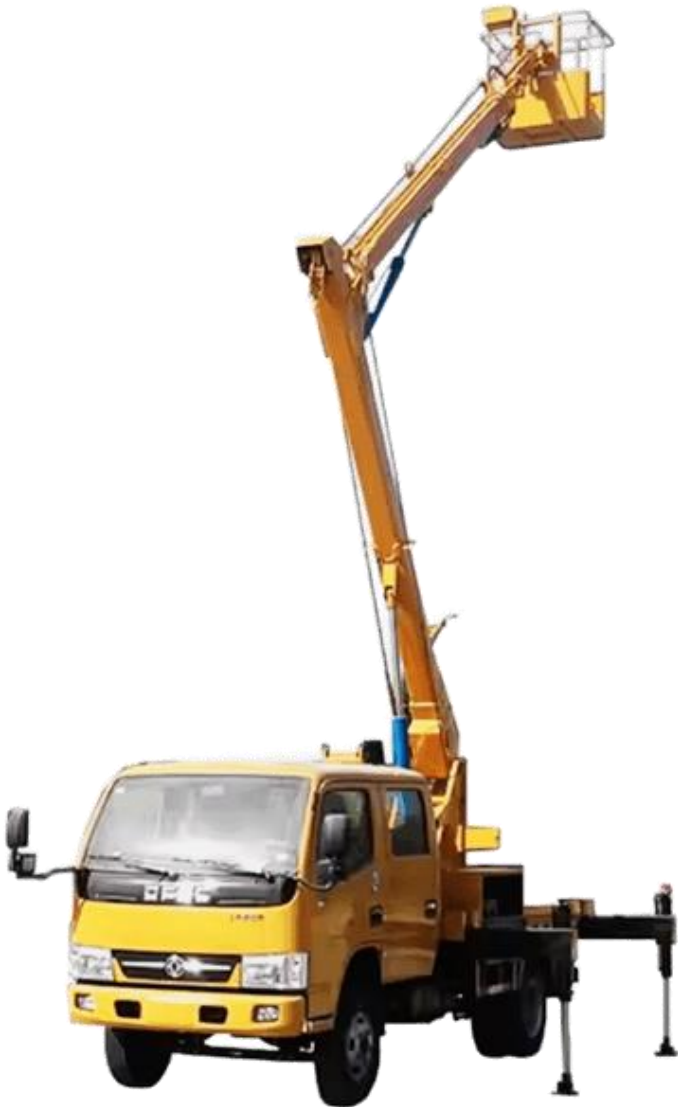
Aerial Work Truck
